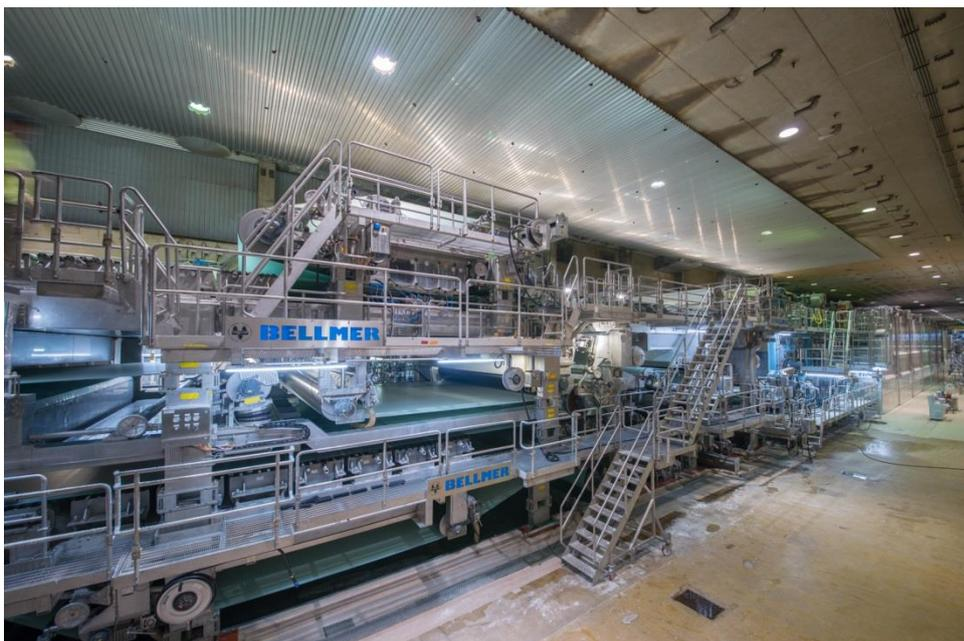
*The new machine with a production capacity of 400,000 t/a*
