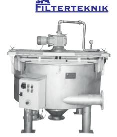
Due to the bottom-up cleaning technique, the BSW gravity strainer achieves an exceptionally high operational reliability and is more effective and efficient in retaining solids and fibres, which results in an improved final filtrate. Large differences in contamination as well as fibrous contaminants are easily handled by the BSW gravity strainer.
